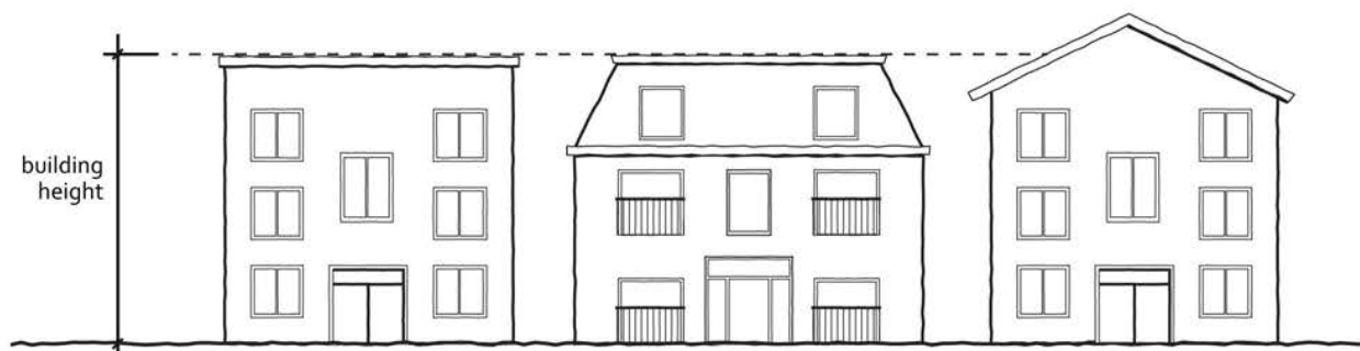
Figure 13-5. Building Height Measurement
