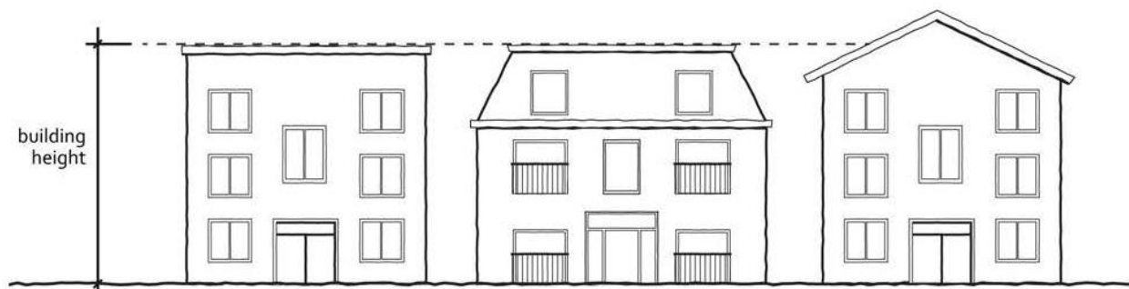
Figure 13-5. Building Height Measurement
