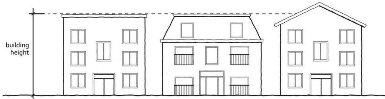
Figure 13-5. Building Height Measurement
