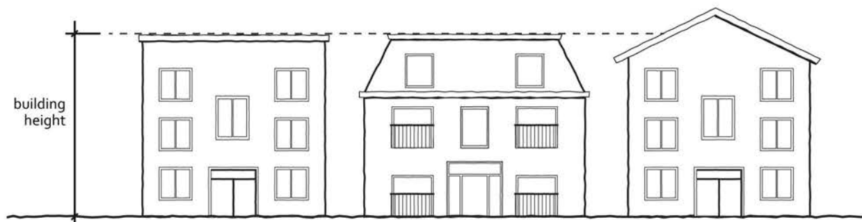
Figure 13-5. Building Height Measurement
