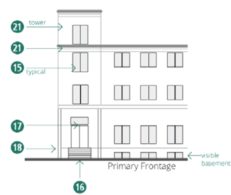
Figure 4-15. Civic Building: Facade Design Requirements
