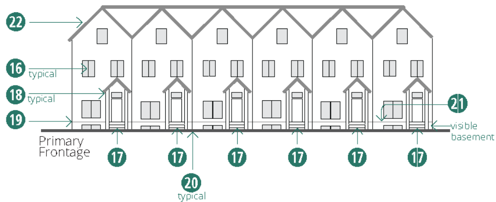
Figure 4-12. Row Building: Facade Design Requirements
