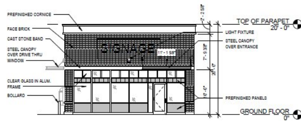
④ SOUTH ELEVATION - ST CHARLES RD 1/8" = 1'-0"
